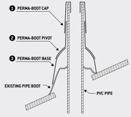
The 3-part system is simple to install and warrantied for the life of the shingles.
